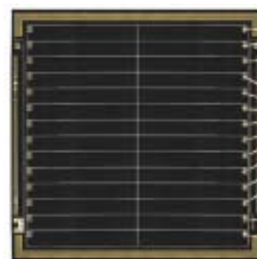
A 14x14 mm 2 wide aperture modulator divided into 28 rectangular pixels
