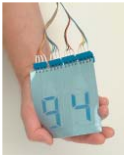
Demonstrator of a seven segment display printed on paper
